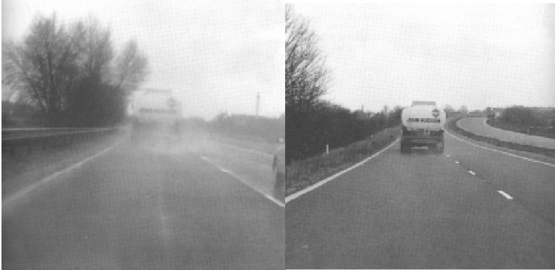
Fig 7: Comparison of spraying generated by a tanker traveling on conventional asphalt (on left) vs. traveling on porous asphalt (on right).
